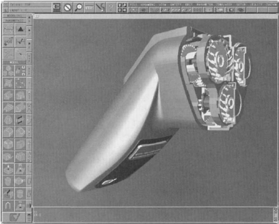
Fig. 13.12 Solid model of an electric shaver design (courtesy of ComputerVision, Inc.).
