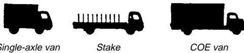
Fig. 11.1.45 Medium- and heavy-duty truck classification by gross weight and vehicle usage. (Reprinted with permission from SAE, SP-868, ©1991, Society of Automotive Engineers, Inc.)
