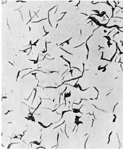
Fig. 6.3.2 Gray iron with flake graphite. Unetched, 100×.
