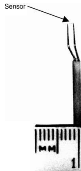
Fig. 20.7.6 Photograph of boundary-layer-type hot-wire probe.
