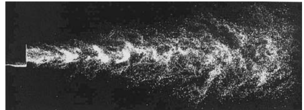
Fig. 20.7.11 Flow structure of a nitrogen jet at Mach 0.6.
