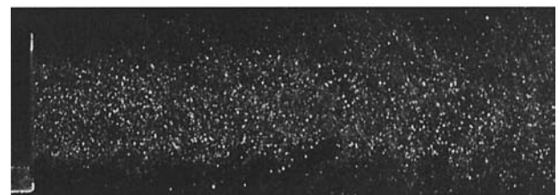
Fig. 20.7.12 Cross-correlation images for nitrogen jet at Mach 0.6.
