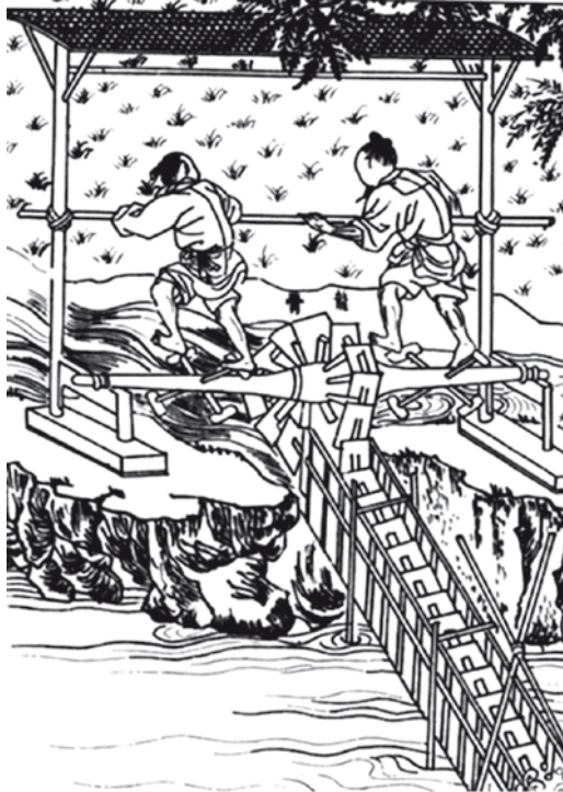
Fig. 2.7 Chain water elevator (From the Thien Kung Khai Wu [86])
