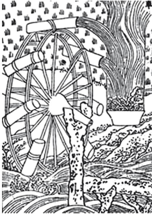
Fig. 2.8 Bamboo water wheel (From the Nong Shu [86,141])
