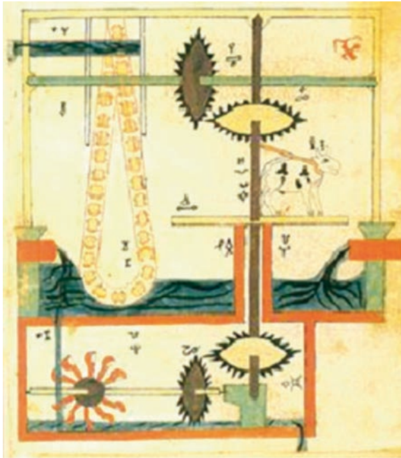
Fig. 4.3 Al-Jazari's water raising device [9]
