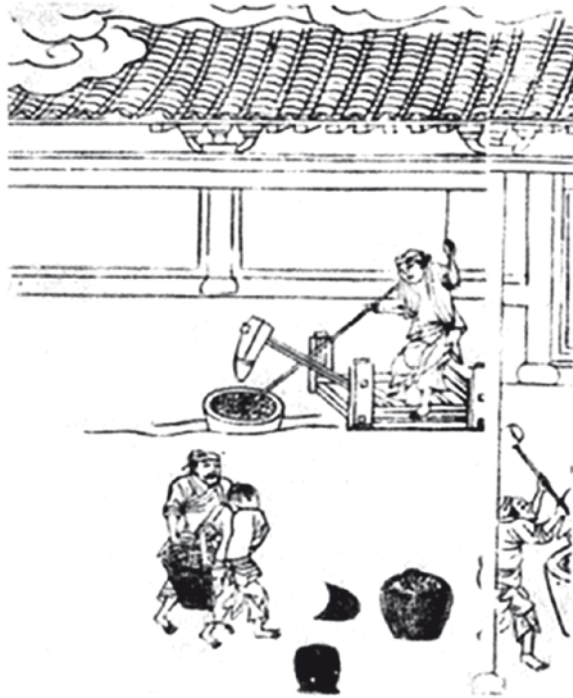
Fig. 2.10 Foot-operated hammer (From the Kêng Chih Thu [86])
