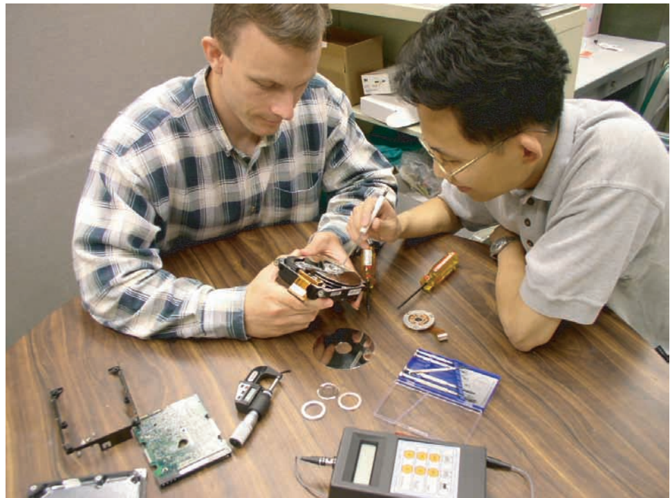
FIGURE 1.36. The construction and function of a device can be learned from its disassembly, examination, and reassembly in a process known as mechanical dissection.
