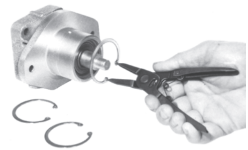
FIGURE 17.45. Internal ring pliers; when the pliers are squeezed, the lugs are compressed toward each other. Courtesy of Koh-I-Noor Rapidograph
