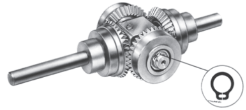
FIGURE 17.43. An external retaining ring used in a precision differential gearset. Courtesy of Koh-I-Noor Rapidograph
