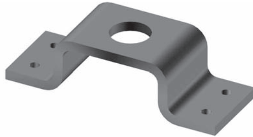
FIGURE 16.66. Profile of a surface also can be used to make sure two or more surfaces are coplanar.
