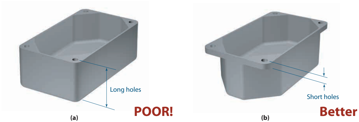
FIGURE 9.52. Long holes such as those on the original part in (a) are difficult to keep straight because drill bits bend more as they cut deeper. When possible, holes should be kept short, as on the redesigned part in (b).
