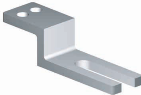
FIGURE 9.49. Using high-volume fabrication methods, what sequence of processes would be needed to create this part?
