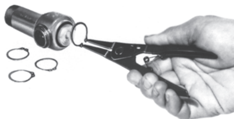
FIGURE 17.46. Internal ring pliers; when the pliers are squeezed, the lugs are spread apart. Courtesy of Koh-I-Noor Rapidograph
