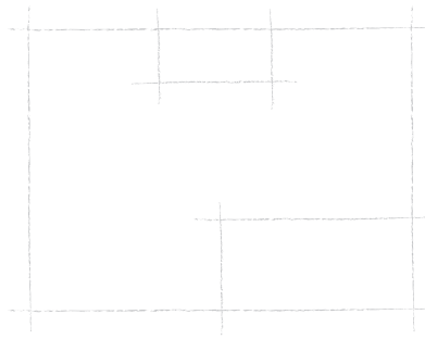
FIGURE 2.10. Construction lines used to create a sketch.
