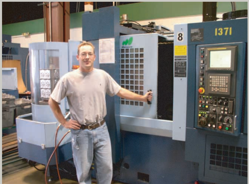
The workpiece is placed in a computer-controlled Matsuura four-axis milling machine, which reduces the workpiece into the 1.3 kg AeroTec product shape.
