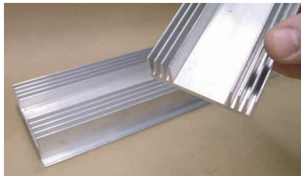
FIGURE 9.28. By changing the shape of the orifice in the extrusion die, custom geometries such as these heat sinks can be created.
