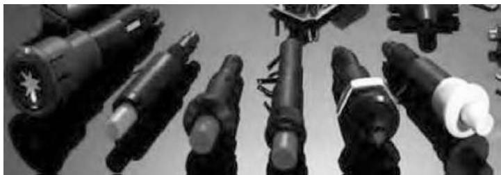
Figure 2-3 Piezoelectric PZT-based gas igniters. When the piezoelectric material is stressed (by applying a pressure) a voltage develops and a spark is created between the electrodes. (Courtesy of Morgan Electro Ceramics, Inc.)
