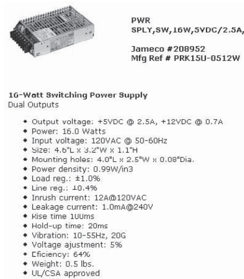
Figure 7.24 Specifications for an example closed-frame power supply.
