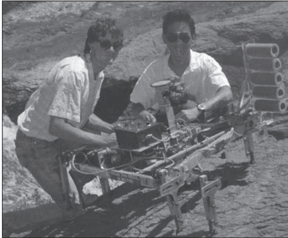
(a) "Lurch"—Scotch yoke mechanism leg design (1989)
