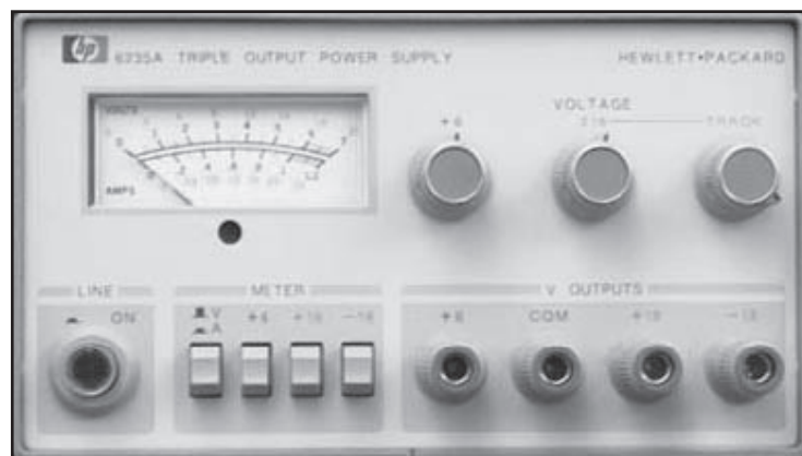
Figure 7.22 Example of a full-featured instrumentation power supply.
