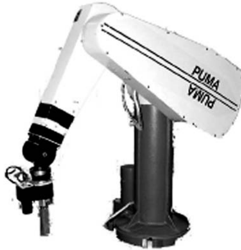
FIGURE 15.2 PUMA with attached gripper and vision module.
