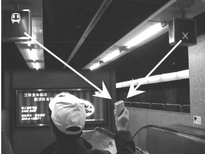
FIGURE 8.5 Application of i.LIGHT to provide platform directional guidance.
