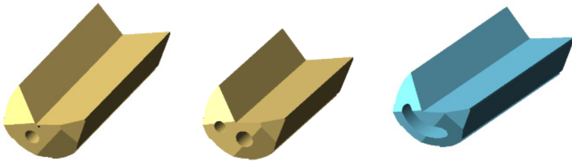
Fig. D.11. Different shapes of the coolant passage adopted by gundrill manufactures: one round hole, two round holes, and a kidney-shaped hole.
