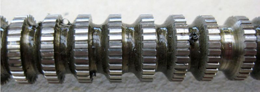
Fig. 3.66. Conventional spline broaching tool
