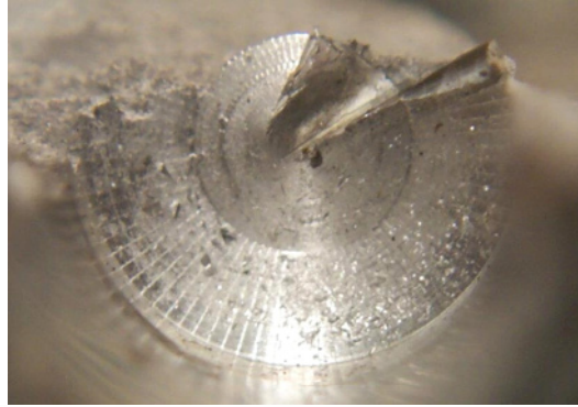
Fig. 3.58. Chatter marks on the bottom of the hole being drilled
