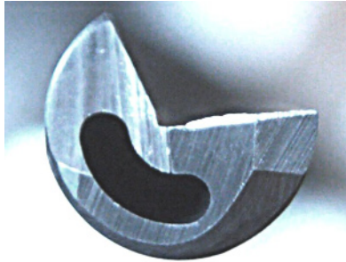
Fig. 5.21. Combined point grind
