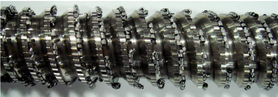
Fig. 3.67. Helical spline broaching tool
