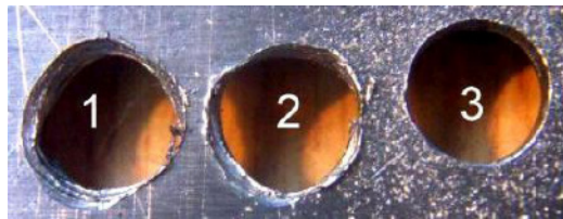
Fig. 4.64. Hole entrances made by a drill with: 1- excessive web eccentricity, 2 – maximum allowable web eccentricity, 3- with web eccentricity less than 1^\circ
