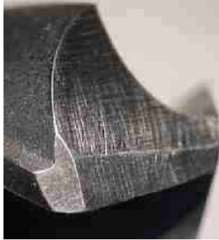
Fig. 4.73. Planar flank face ground on the top of a standard conical grind
