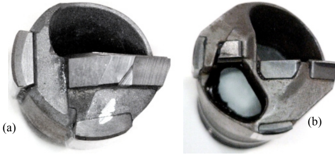
Fig. 5.6. Drill design: (a) with single cutting insert, and (b) with partitioned cutting edge made by three cutting inserts
