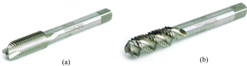
Fig. 3.65. Two basic threading tap designs with the cutting edge inclination angle
