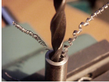
Fig. 4.65. Unequal chips from the lips
