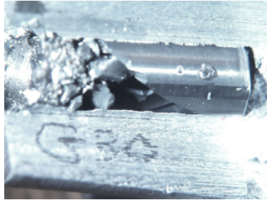
Fig. 5.15. Gundrill failure due to chip clogging
