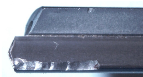
Fig. 5.50. Bulk fracture of the side cutting edge
