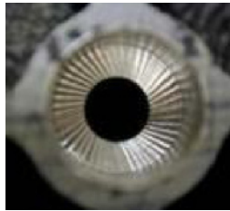
Fig. 3.59. Chatter marks on the bottom of the hole being engraved with a twist drill
