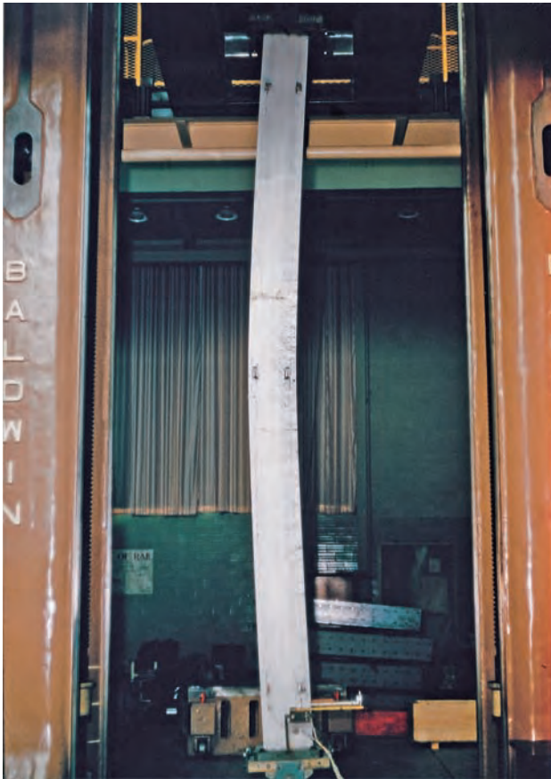
Photo 10.1 Laboratory test showing a buckled column.
