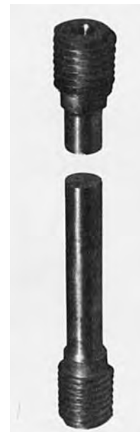
Photo 2.5 Tested specimen of a brittle material.
