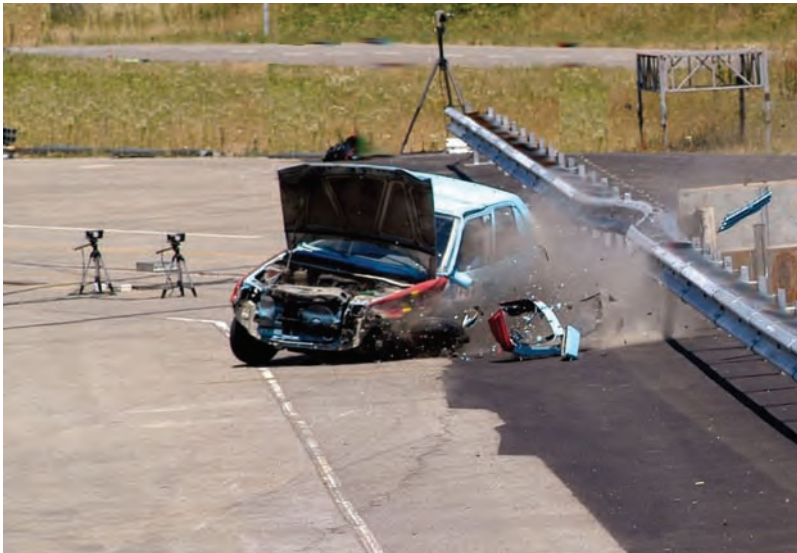
Photo 11.3 As the automobile crashed into the barrier, considerable energy was dissipated as heat during the permanent deformation of the automobile and the barrier. Source: Crash test photo courtesy of Sec-Envel and L.I.E.R., France.
