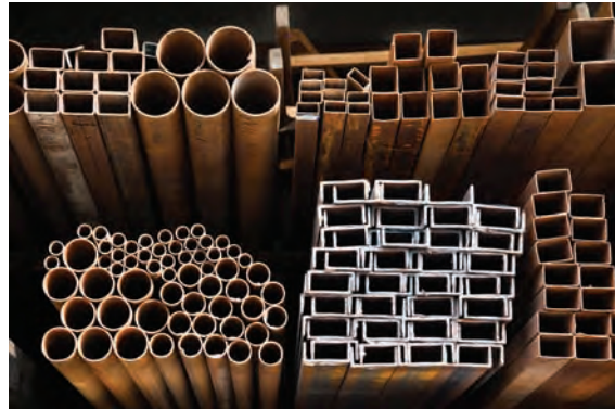
Photo 6.3 Box beams and tubes.
