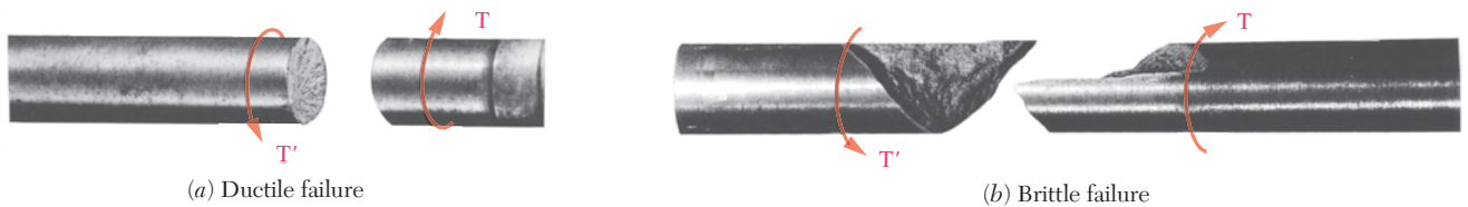
Photo 3.2 Shear failure of shaft subject to torque.
