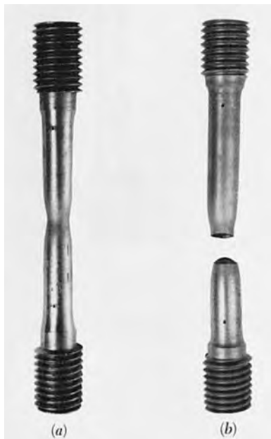
Photo 2.4 Tested specimen of a ductile material.
