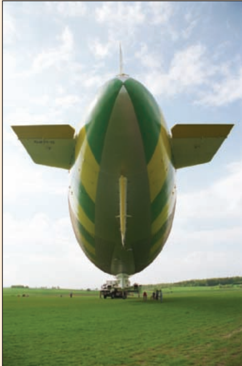
Airships such as this blimp rely on internal pressure to maintain their shape using a gas lighter than air for buoyant lift. (Courtesy of Christian Michel, www.modernairships.info )
