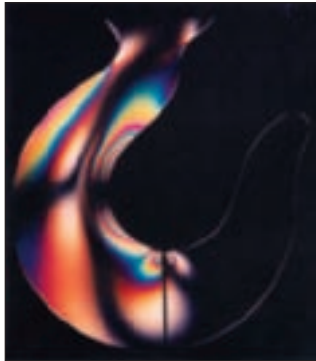
(b) Photoelastic fringe pattern (Courtesy of Eann Patterson)
