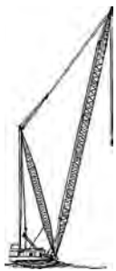
Fig. 10.4.29 Ringer crane. (Construction Safety Association of Ontario.)
