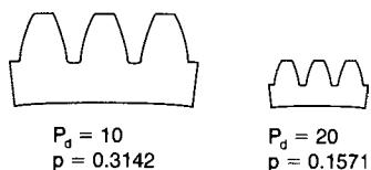
Fig. 8.3.1b Comparison of pitch and tooth size.
