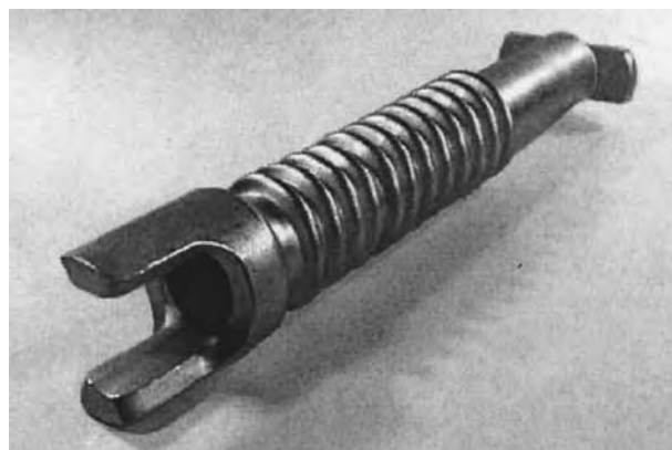
Fig. 13.2.30 Automotive steering column manufactured by cold-forging aluminum alloy. (Source: N. Bay, Cold Forming of Aluminum—State of Art. Jour. Mater. Processing Technol. , 71, 1997, pp. 76–90.)
