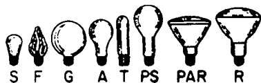
Fig. 12.5.3 Typical filament lamp shapes: S, straight; F, flame; G, globe; A, general service; T, tubular; PS, pear shape; PAR, parabolic; R, reflector.
