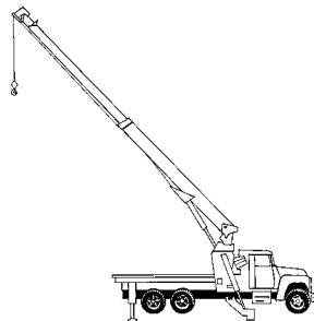
Fig. 10.4.24 Boom truck. ( Construction Safety Association of Ontario. )
