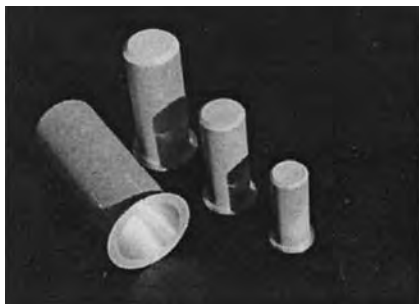
Fig. 11.6.35 SwRI’s inhibited shaped-charge launcher. Various size charges are available that are capable of launching 0.25 to 2 g aluminum projectiles up to 11.5 km/s (left view). Projectiles are typically in the shape of a hollow cylinder (right view.)
