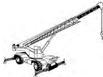
Fig. 10.4.26 Rough terrain crane. ( Construction Safety Association of Ontario. )
