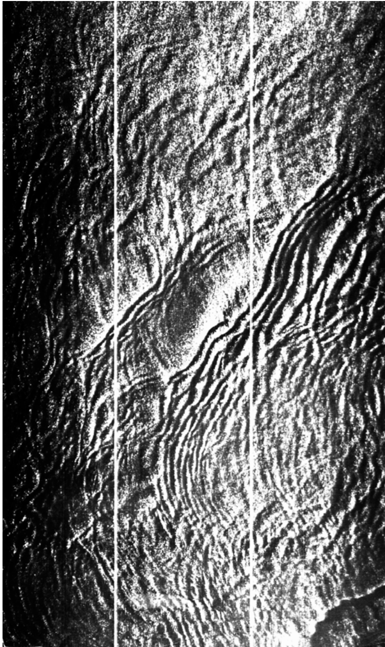
Figure 8.1. Side-looking radar survey experimental pictures of a disturbed sea surface in the Pacific Basin near the Kamchatka Peninsula. The radar survey was carried out by “TOROS” side-looking radar onboard the Russian airplane laboratory AN-24. (a) The radar image indicates the surface manifestations of internal waves in the form of diverging waves positioned in the middle of a sea. The space interval between the white lines is equal to 5 km.
