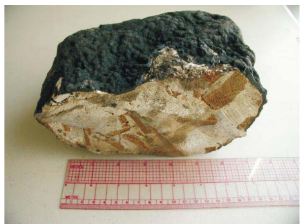
Figure 5 Photograph of a ferromanganese crust on a phosphorite substrate recovered from the summit of Schumann seamount, north of Kauai, Hawaii. Note the inclusions of altered basalt clasts from the seamount within the phosphorite, which has likely replaced limestone. (From G. McMurtry and D. L. VonderHaar, unpublished data.)
