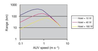
**Figure 2** Range as a function of hotel load and speed. These calculations were made for a low drag 2.2 m long, 0.6 m diameter vehicle with high efficiency propulsion and batteries providing  $3.3 \text{ kW} \cdot \text{h}$  of energy
