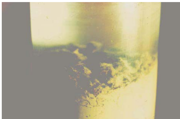
Figure 7 Example of a core tube taken with the SMBA Multi-corer to show the layer of phytodetritus lying on top of the older sediment. This was taken in May 1981 from a depth of 2000 m in the north-east Atlantic.
