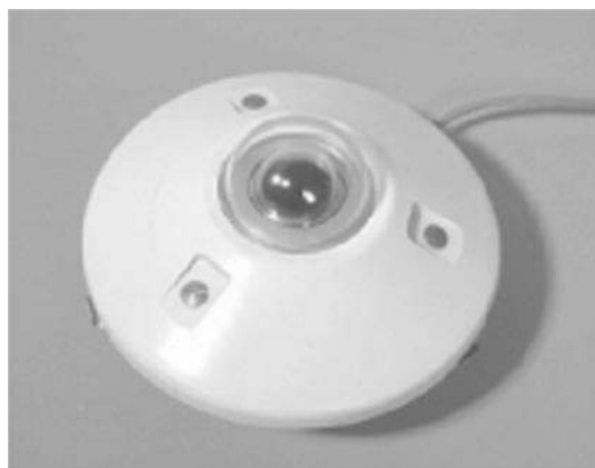
Figure 1 A pyranometer used for measuring short-wave radiation. The thermopile is covered by two transparent domes. (Photograph courtesy of Southampton Oceanography Centre.)
