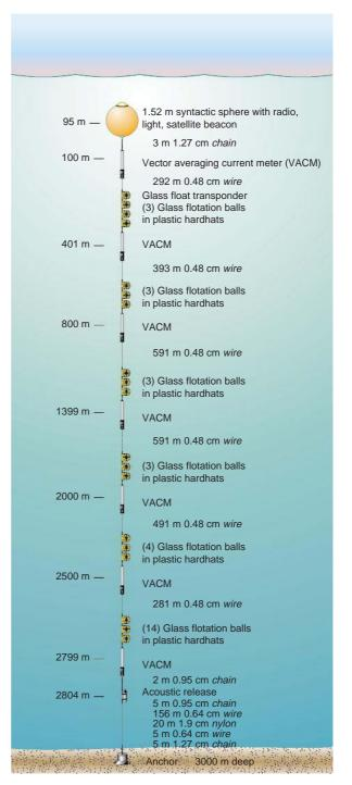
Figure 1 A typical subsurface mooring design. (Design by S. Worrilow.)
