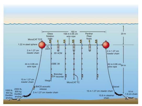
Figure 9 A two-dimensional moored array. (TCP, Temperature, Conductivity and Pressure; BACS, Binary Acoustic Command System; SBE, SeaBird Electronics; ACM, Acoustic Current Meter; Ax Pack, Acceleration package. Design by R. Trask.)
