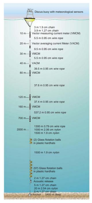
Figure 2 A semitaut surface mooring design. (Design by P. Clay.)
