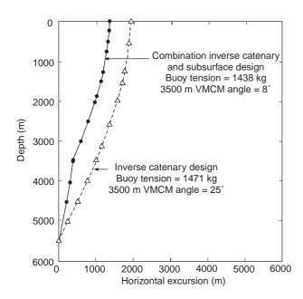
**Figure 6** A comparison of the shapes of two mooring designs subjected to the same ocean current forcing, showing the differences in mooring inclination at 3500 m depth.
