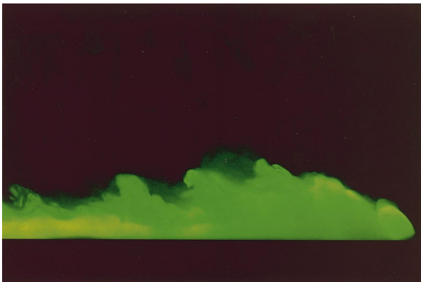
Figure 1 A vertical cross-section showing the structure of the flow in and behind the head of a gravity current advancing over a rigid bottom in a laboratory experiment, from left to right. The dense fluid has been marked by fluorescein dye. Note the dense fluid layer on bottom at the left, and the mixed layer above it. (Dyed salt water inflow density 1.05 \text{ g cm}^{-3} into fresh water, current depth of order 1–2 cm.)
