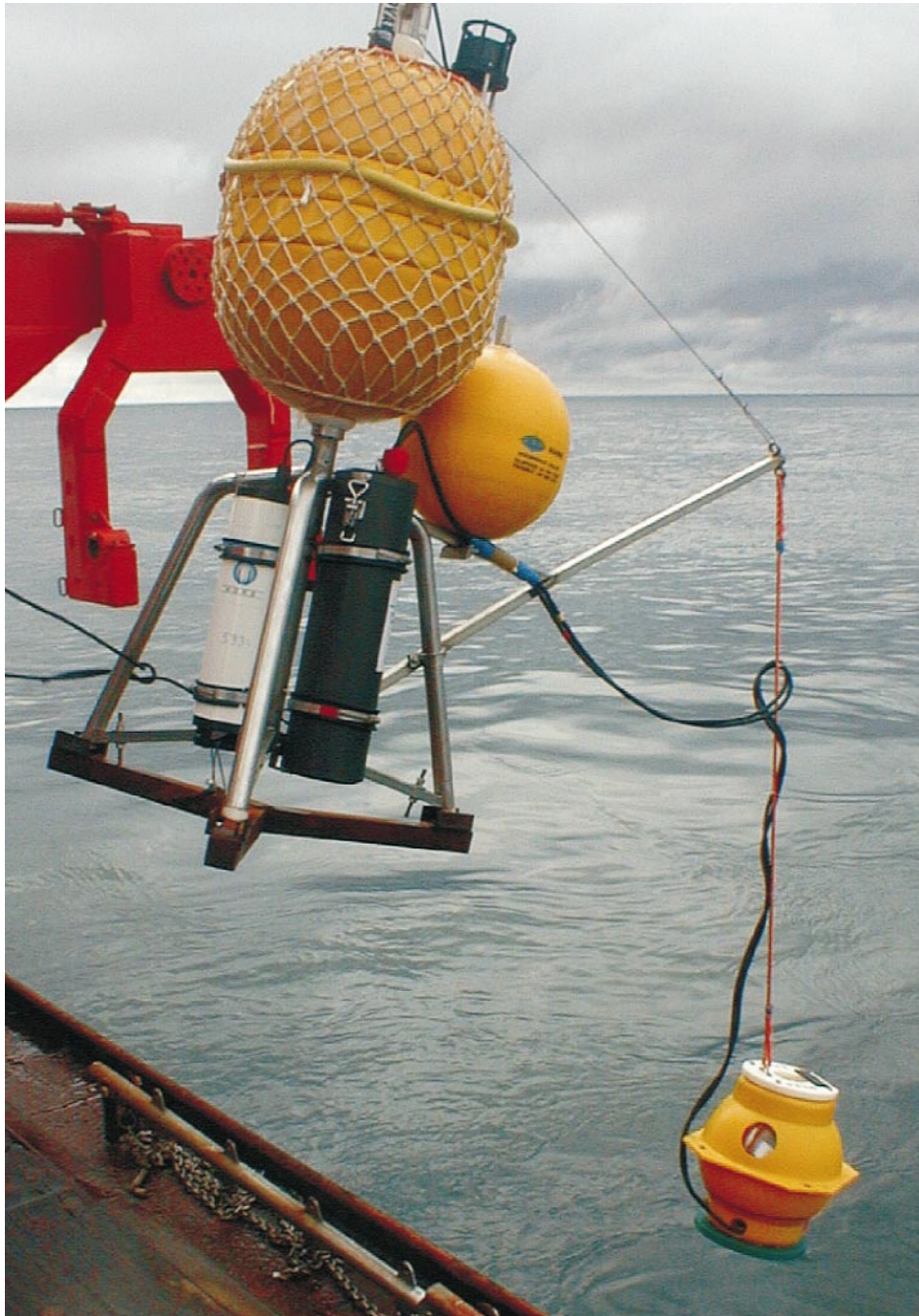
Figure 4 The GEOMAR OBH/S. The shipping/storage container is equipped with an overhead rail so that it serves as an instrument dispenser. The OBS version is shown here. (Photograph by Michael Tryon, UCSD.)
