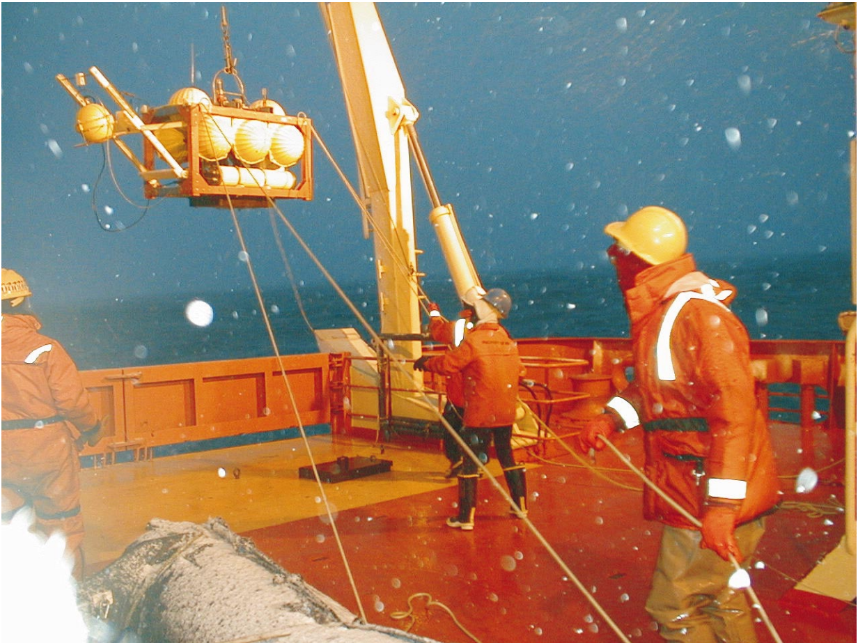
Figure 5 The SIO-ONR OBSs (Jacobson et al. 1991, Sauter et al. 1990) being launched in Antarctica. The anchor serves as a collector for the CAT fluid fluxmeter (Tryon et al. 2001). The plumbing for the flowmeter is in the light-colored box at the right-hand end of the instrument. (Photograph by Michael Tryon, UCSD.)
