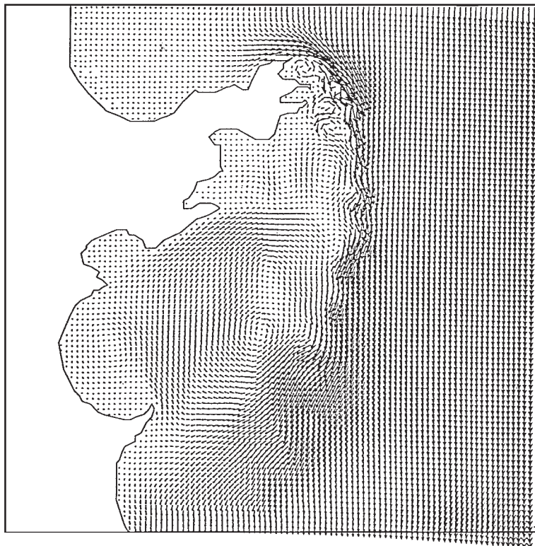
Figure 2 Attached eddies and vortex street in the wake of Bass Point as simulated by a computer model. (Reproduced from Dennis et al. , 1995.) The domain width is 6.67 km, and the maximum current vector, as indicated by the longest arrow, is 0.42 \text{ m s}^{-1} .
