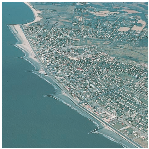
(b) Groins built at right angles to the shore at Cape May, New Jersey, to slow the migration of sand. The groins interrupt the flow of long-shore currents, so sand is trapped on their upcurrent sides. This view is toward the south, and south of the groins, on the downcurrent sides, sand is eroded.
