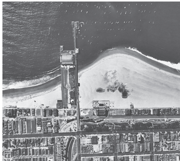
(b) The same shoreline in 1949 after the breakwater was built. The boat anchorage formed by the breakwater is filling with sand deposited by disruption of the long-shore current.
