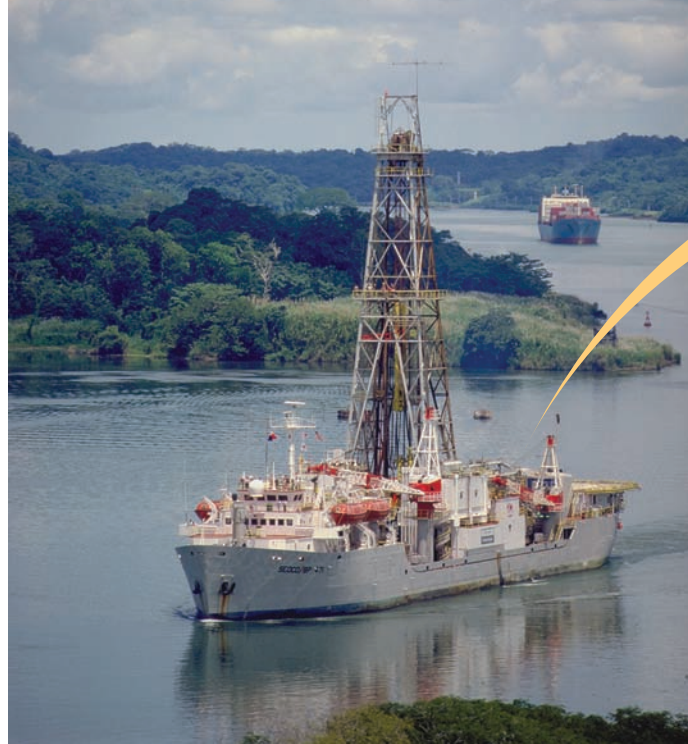
(a) JOIDES Resolution , the deep-sea drilling ship operated by the Joint Oceanographic Institutions for Deep Earth Sampling. The vessel is 124 meters (407 feet) long, with a displacement of more than 16,000 tons. The rig can drill to a depth of 9,150 meters (30,000 feet) below sea level.
