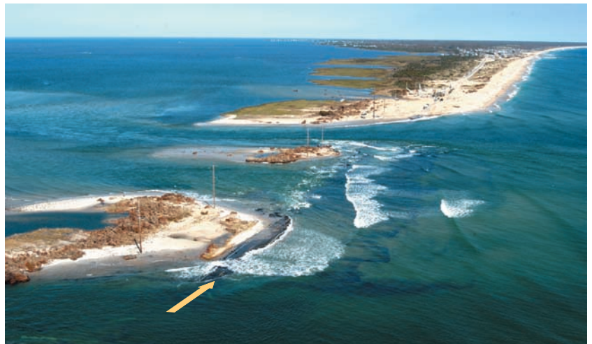
(b) This breach of Hatteras Island on North Carolina's outer banks was caused by storm surge and flooding by Hurricane Isabel in September 2003. The ocean is to the right.
