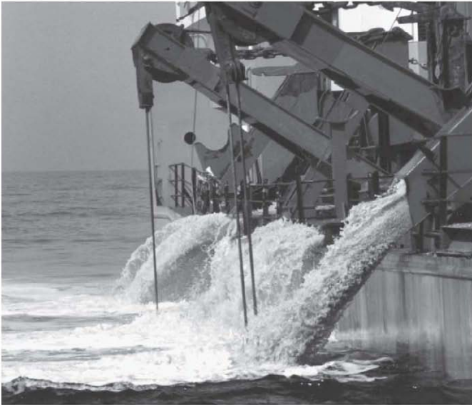
Fig. 1. Discharge of overflow and screened.
