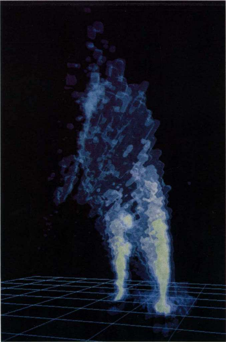
Plate 3 Three-dimensional reconstruction of two hydrothermal plumes emanating from black smoker-type sea-floor hot springs. Data obtained at sound frequency 330 kHz. (P. A. Rona et al, "Acoustic imaging of hydrothermal plumes," Geophy. Res. Ltrs. 18 [12], 2233-36 [1991]).
