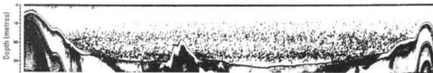
Figure 10.1.2 A nighttime 70 kHz echo sounding record taken in Trout Lake, Wisconsin. Some of the bottom echoes saturate the receiver electronics and cause the trace to be white. (From Rudstam, L. G., C. S. Clay, and J. J. Magnuson, “Density estimates and size of cisco, Coregonus artedii , using analysis of echo peak PDF from a single transducer sonar,” Can. J. Fish. Aquat. Sci. 44 , 811–21, 1987.)
