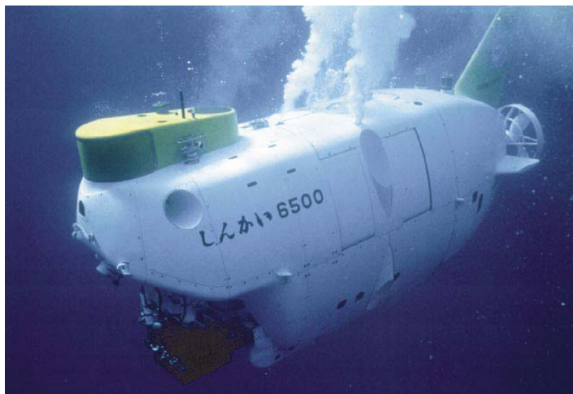
Figure 9 Japanese 6000 m-class submersible Shinkai 6500 .
