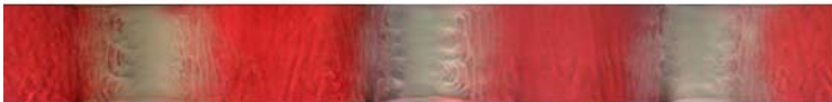
Plate 10.4: Top view of a sandy bed under a standing wave after four days. Initially the bed is a pink layer of sand mixture of two diameters: 0.2 mm (red) and 0.11 mm (light), in roughly equal parts. Periodic bands of coarse (red) and fine (light) sands are eventually found beneath wave nodes and antinodes. Experiments and photograph by Blake Landry and Matthew Hancock, Dept. Civil & Environ. Eng., MIT, 2003.
