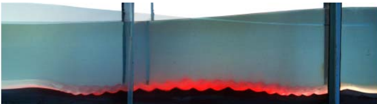
Plate 10.3: Side view of a sandy bed under a standing wave after four days. Initially the bed is a pink layer of sand mixture of two diameters: 0.2 mm (red) and 0.11 mm (light), in roughly equal parts. Eventually coarse (red) sand is accumulated beneath the node where ripples and a bar crest are formed. Beneath antinodes, the bed is flat and is covered by fine (light) sand. Experiments by Blake Landry and Matthew Hancock, Dept. Civil & Environ. Eng., MIT. Photograph by Felice Frankel, MIT, 2003.
