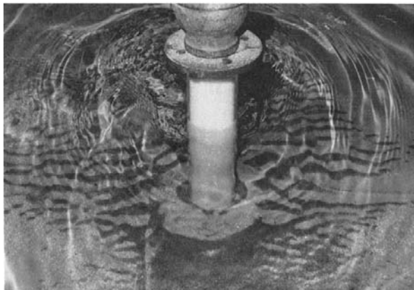
Plate 10.5: Sediment accumulation (see dark areas) near two sides of a circular pile. Wave crests are parallel to the ripple marks. Prior to wave motion, there were no sand particles in an annular area next to the cylinder (from Lamoure and Mei, 1977, J. Fluid Mech. Reproduced by permission of Cambridge University Press).
