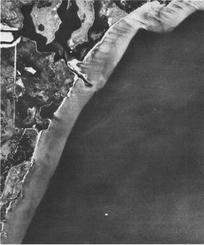
Plate 10.1: Aerial view of submarine longshore bars Escambia Bay, Florida (from Lau and Travis, 1973, J. Geophys. Res. Reproduced by permission of American Geophysical Union).
