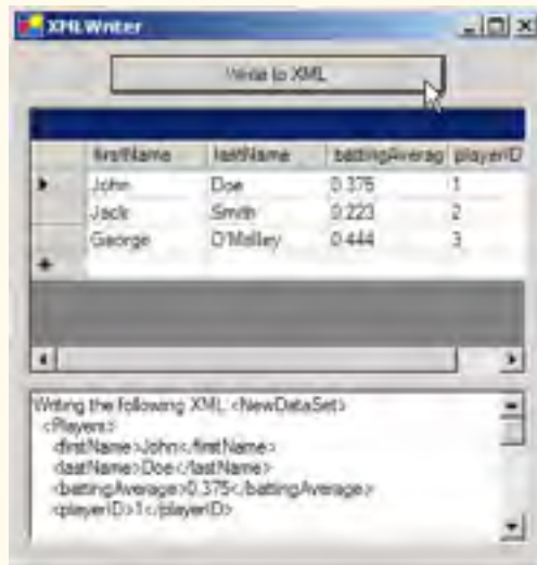
Fig. 19.30 Application that writes an XML representation of a DataSet to a file.
