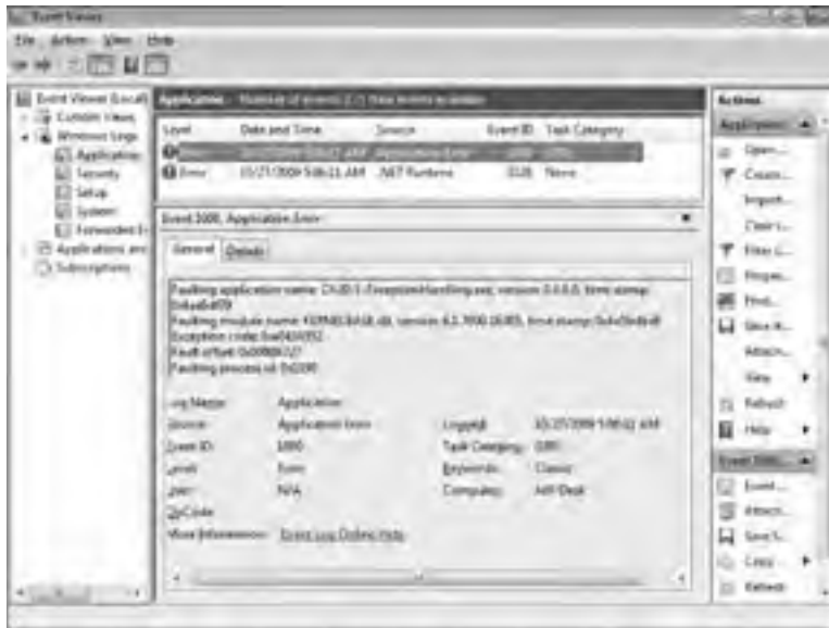
FIGURE 20-1 Windows Event log showing an application that terminated due to an unhandled exception
