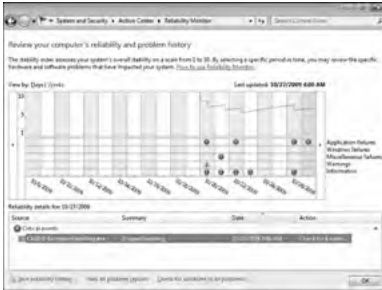
FIGURE 20-2 Reliability Monitor showing an application that terminated due to an unhandled exception
