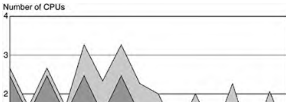
Figure 3-4. Utilization after consolidation—50% utilization of four CPUs
