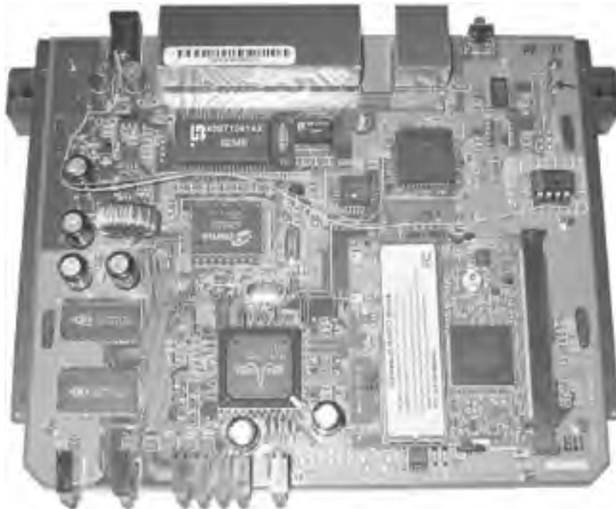
The last requirement was to add a DB9 connector so we could connect to the serial port with a laptop. For this, we needed pins 2, 3, and 5 from the pinout marked UART2. It is important to note that unlike a standard RS-232 DB9 pinout, pins 2 and 3 are not crossed. The pinout to the DB9 is as follows:
