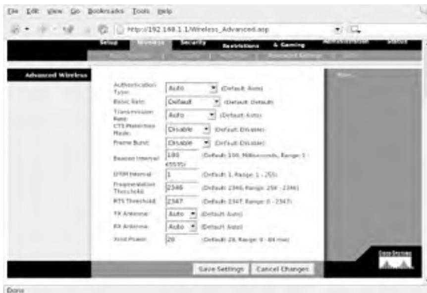
If you have two WRT54G units, a Linux box with a Prism card and the HostAP driver, or an access point running the OpenAP/LinuxAP distributions (see [Section 6.3.4](#) later in this chapter), you have the option of setting up WDS between your access points. If you choose to use a Prism card, it must have station firmware Version 1.50 or higher. See [Chapter 4](#) for details on how to determine your station firmware version.
