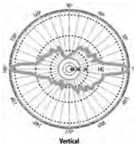
While the theoretical beamwidth of an omnidirectional antenna is 360 degrees horizontally, the vertical beamwidth of most omni antennas is less than 8 degrees. See [Figure 1-9](#) for a side view of a typical omni antenna. Notice that if the antenna were mounted high enough, someone directly under the antenna itself would have very poor signal quality.
