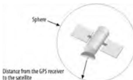
To pinpoint your exact location, GPS uses at least three satellites to triangulate an exact location on earth. [Figure 10-3](#) shows that if you have two satellites, then you can narrow down your location to the intersection of the two spheres. In this case, you can be anywhere on the dotted line (which is an ellipse).
