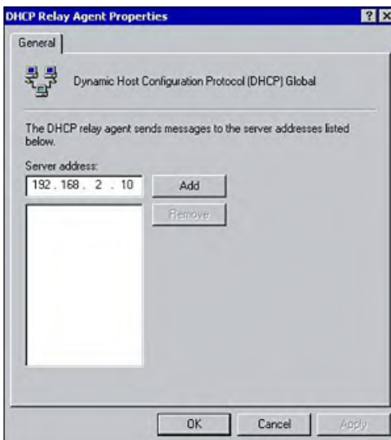
Figure 4.11. Configuring the RAS server with the IP address of the DHCP server.
