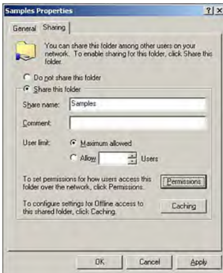
Figure 2.1. Creating a network share by accessing the Sharing tab of a folder's properties sheet.
