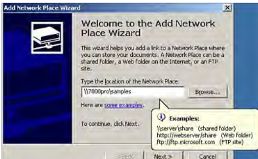
Figure 2.2. Connecting to a shared network folder with the Add Network Place Wizard.
