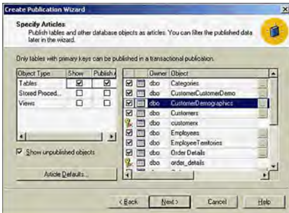
Figure 22.27. The Specify Articles screen allows you to choose which tables you are going to publish.
