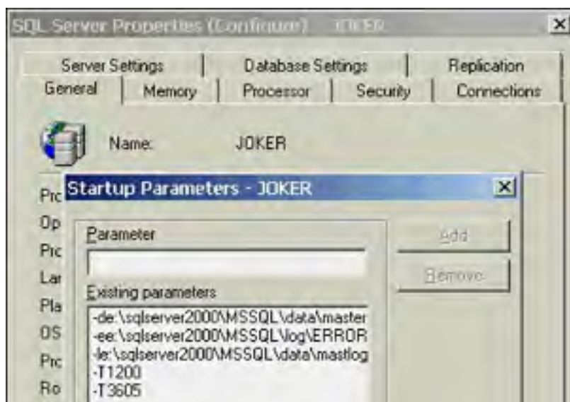
Figure 38.16. Setting the 1200 and 3605 trace flags to be enabled on SQL Server startup.
