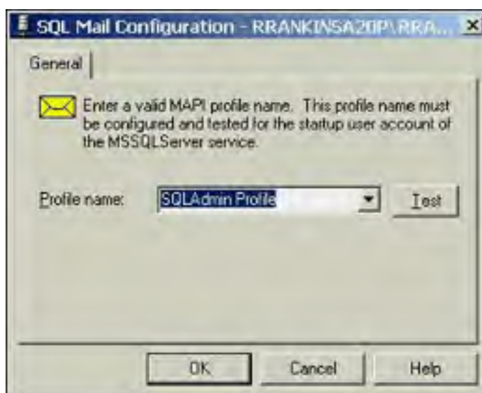
Figure 23.2. Choosing the mail profile for SQL Mail in the SQL Mail Properties dialog box.
