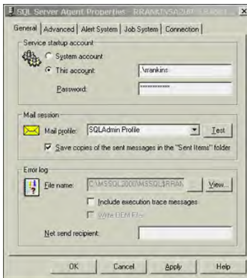
Figure 23.4. Specifying the mail profile to be used by SQLAgentMail in the SQL Server Agent Properties dialog box.
