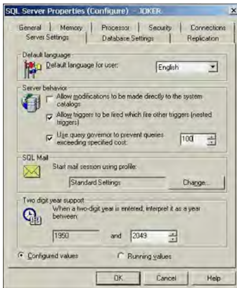
Figure 35.20. Configuring the Query Governor settings in the SQL Server Properties dialog box.
