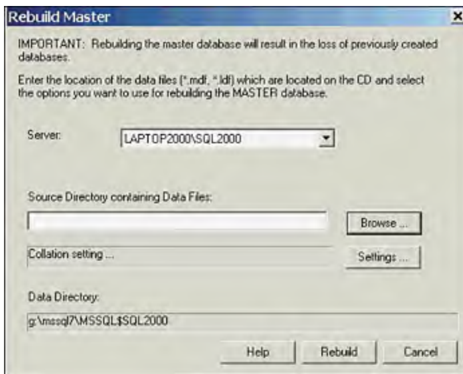
Figure 16.9. The Rebuildm.exe interface.
