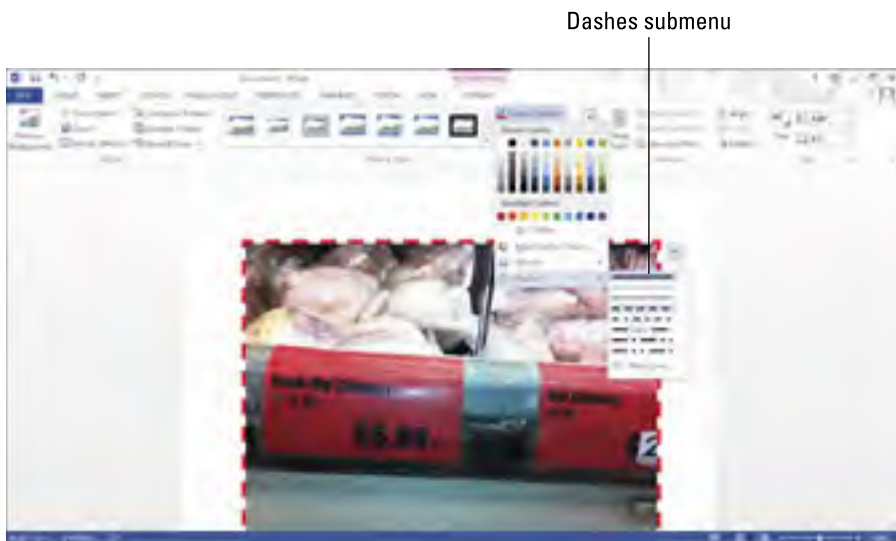
Figure 3-11: The Dashes submenu lets you define the line used to create a border.
