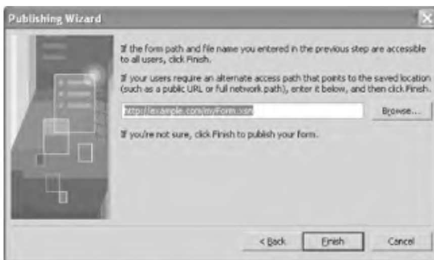
Figure 10-12. Final step of the publishing wizard, where the publishUrl attribute is set
