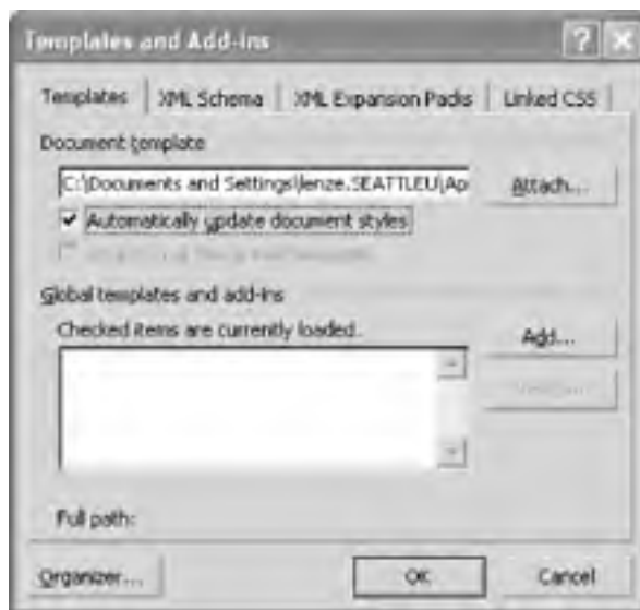
Figure 2-27. The "Automatically update document styles" checkbox
