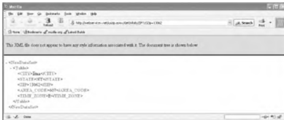
Figure 9-16. A test invocation of the web service using GET
