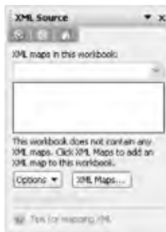
Figure 6-20. The XML Source task pane, before any sources are listed
