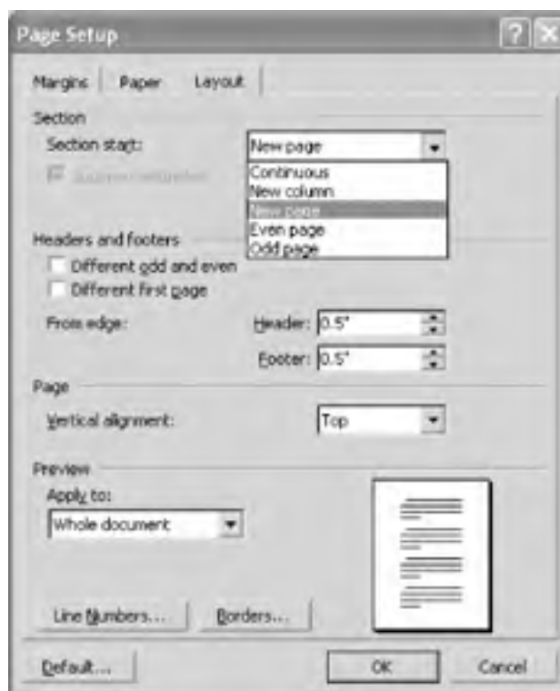
Figure 2-19. The Page Setup dialog for section settings
