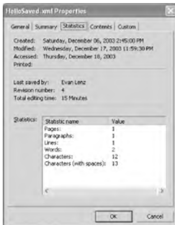
Figure 2-3. The Statistics tab of the Properties dialog, corresponding to values inside the o:DocumentProperties element
