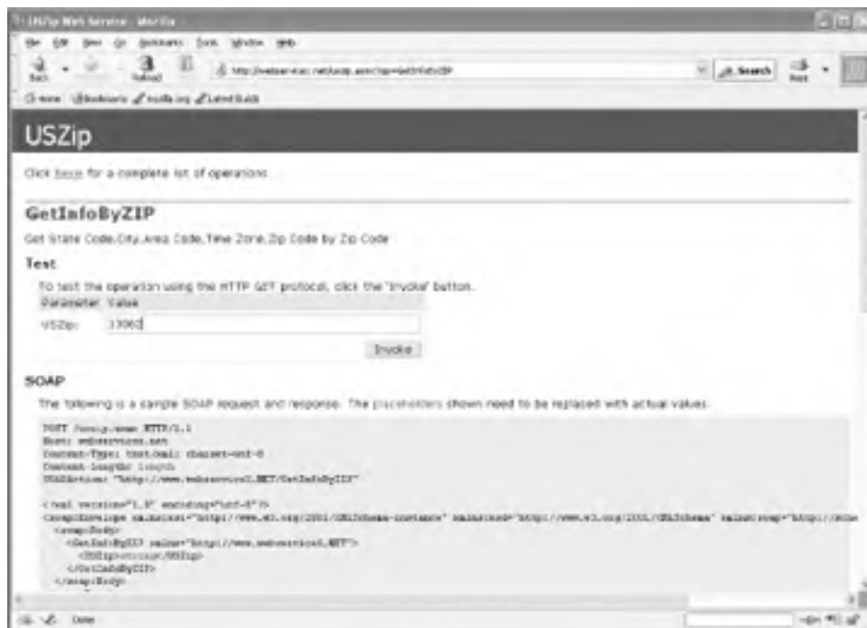
Figure 9-15. Test form that supports the web service
