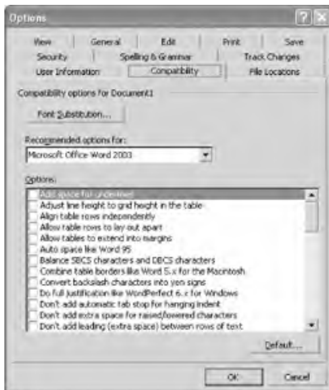
Figure 2-6. Compatibility options, corresponding to the child elements of w:compat
