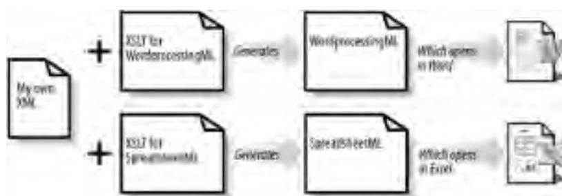
Figure 1-5. Using XSLT to generate WordprocessingML or SpreadsheetML from a custom XML vocabulary
