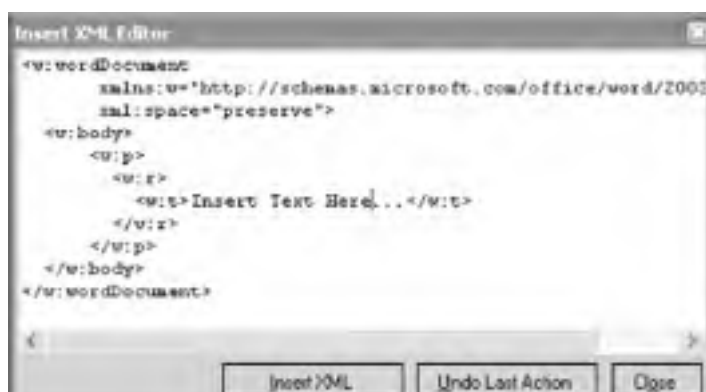
Figure 2-2. The "Insert XML" dialog, available only with the XML Toolbox plug-in for Word
