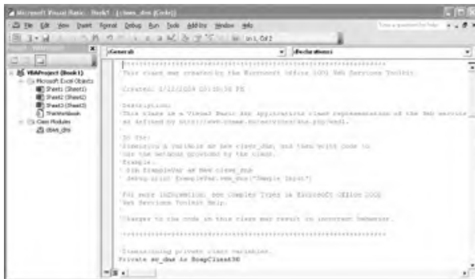
Figure 9-4. VBA code for accessing the DNS service generated by the Web Services Toolkit
