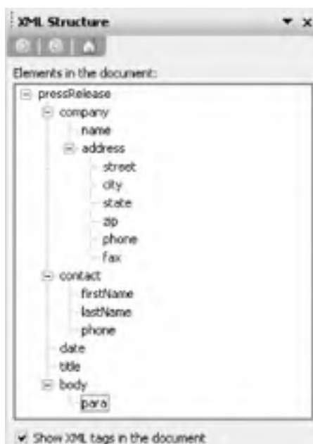
Figure 4-34. The XML Structure task pane with "Ignore mixed content" turned on
