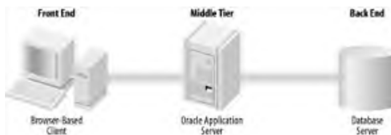
Figure 1-1. Typical three-tier configuration with Oracle Application Server
