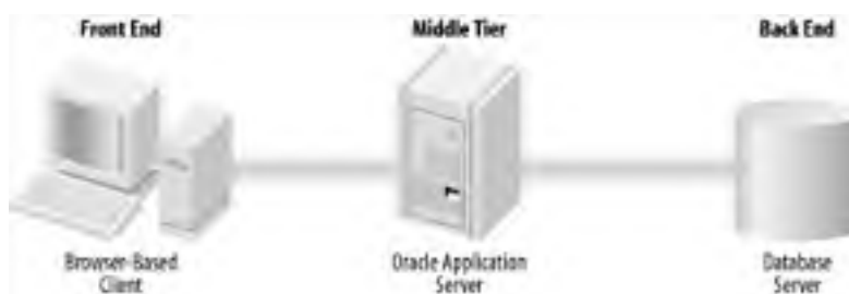
Figure 1-1. Typical three-tier configuration with Oracle Application Server
