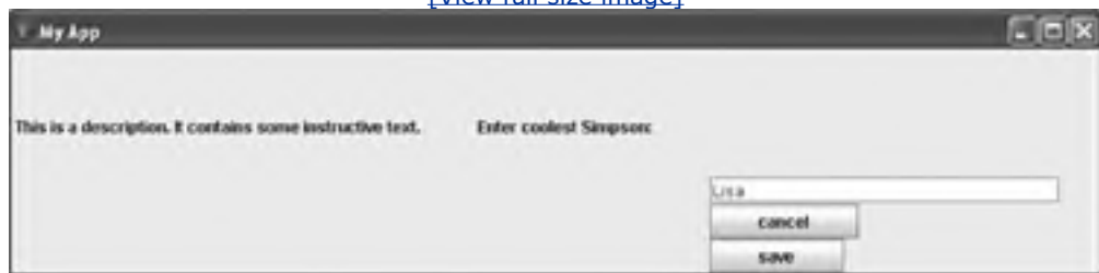
Figure 25.7. The grid bag layout in action.
