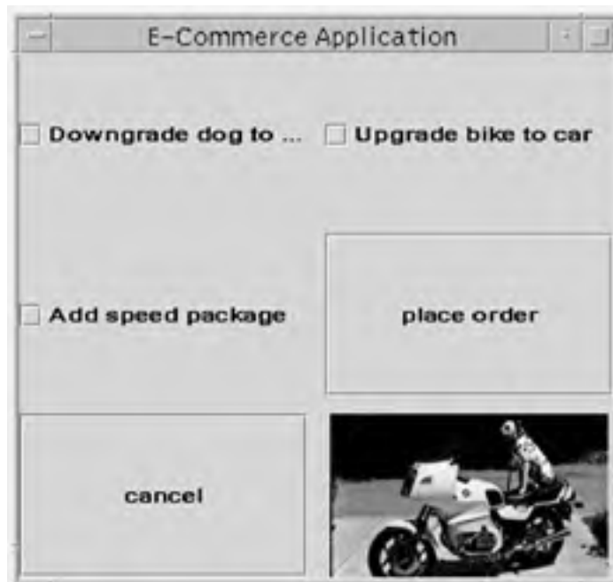
Figure 22-7. A grid layout puts things in equal-sized boxes starting from the top left
