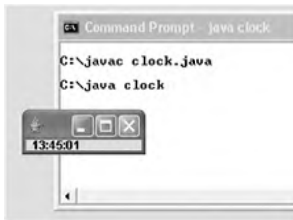
Figure 2-4. Compiling and running the clock program
