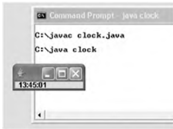
Figure 2-4. Compiling and running the clock program
