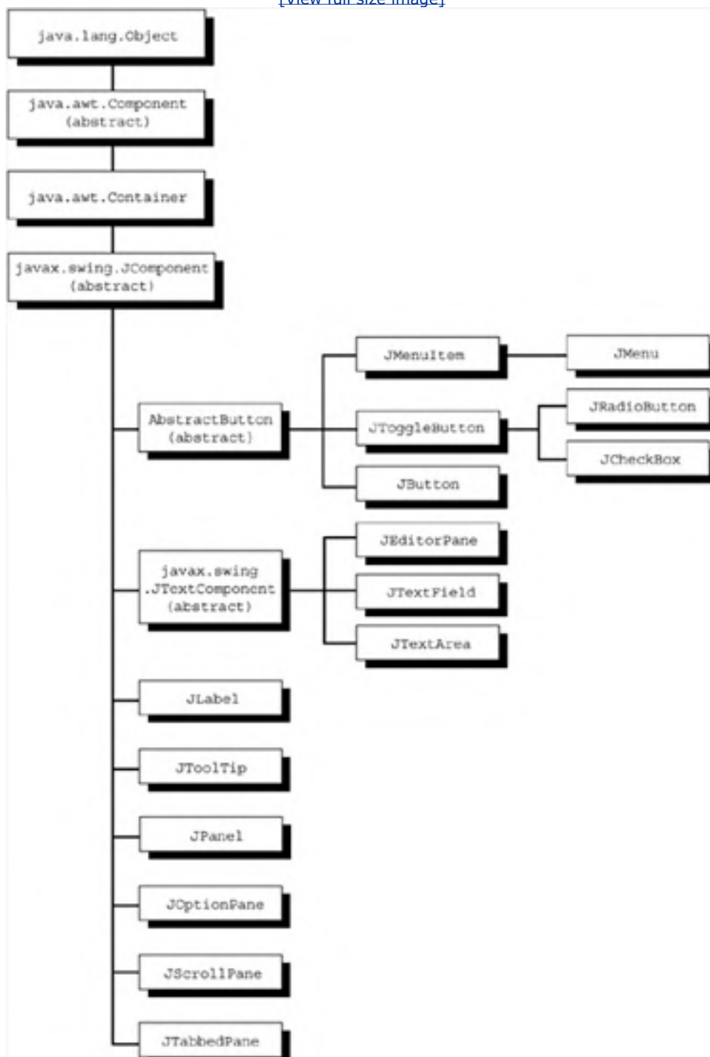
Figure 21-1. Some JComponent controls (visible GUI objects) of Java
