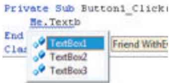
Figure 5-9 Getting help from IntelliSense by typing a period (.) after a valid object
