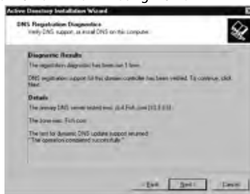
Figure 4.26 The DNS Registration Diagnostics Dialog Box Used for a New Child Domain in an Existing Domain
