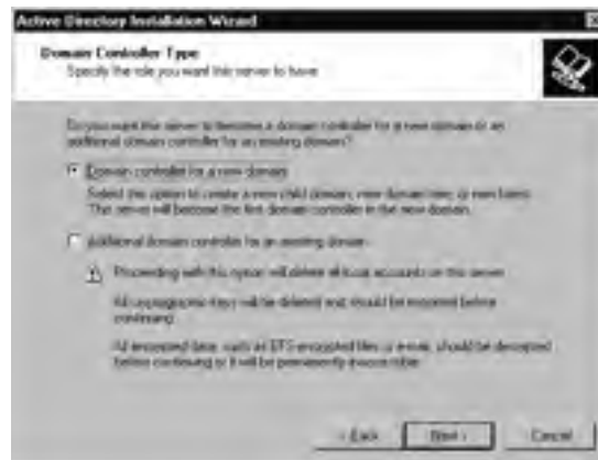
Figure 4.6 The Domain Controller Type Dialog Box Used for a New DC in a New Domain
