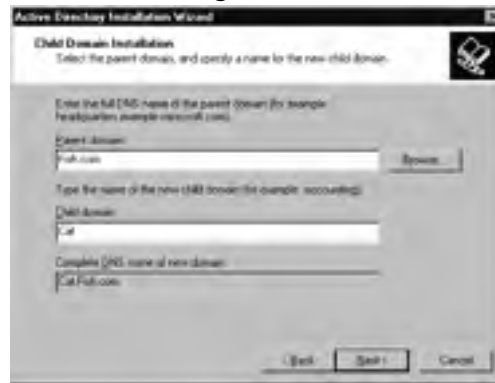
Figure 4.25 The Child Domain Installation Dialog Box Used for a New Child Domain in an Existing Domain
