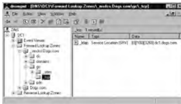
Figure 4.16 The DNS Administrator Tool Used to Verify a Successful Forest-Root Installation
