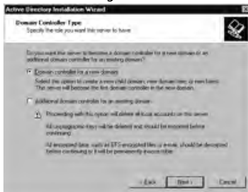
Figure 4.23 The Domain Controller Type Dialog Box Used for a New Child Domain in an Existing Domain
