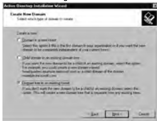
Figure 4.19 The Create New Domain Dialog Box Used for a New Domain Tree in an Existing Forest
