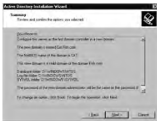
Figure 4.27 The Summary Dialog Box for a New Child Domain in an Existing Domain
