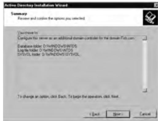
Figure 4.32 The Summary Dialog Box Used for an Additional DC in an Existing Domain
