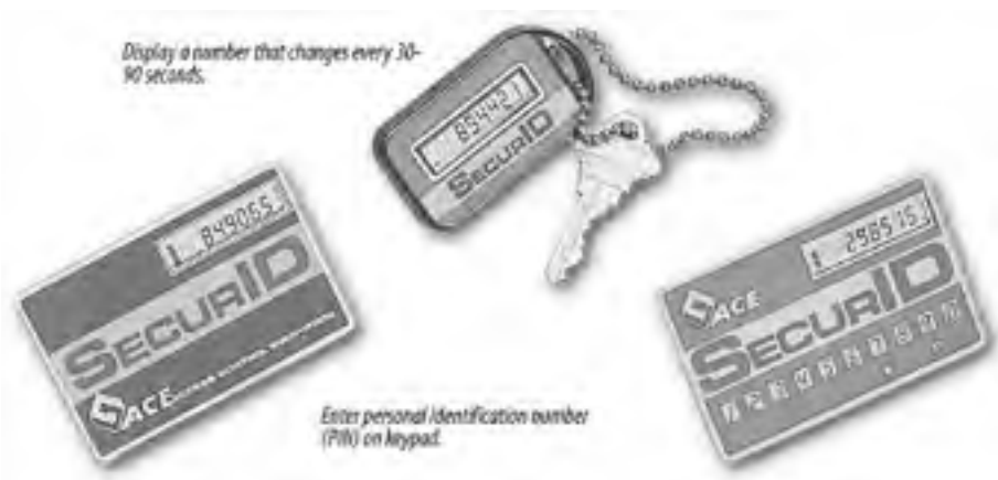
Figure 19-3. Security Dynamics SecurID cards and fob
