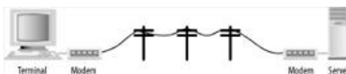
Figure 10-2. A terminal and a computer connected by two modems
