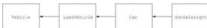
Figure 8.2: The arrows in this diagram represent the direction from which classes can access other classes.
