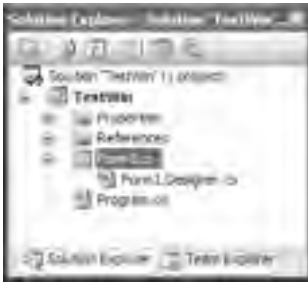
Figure 19-10. Each Form is composed of two *.cs files.
