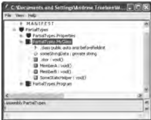
Figure 4-14. Once compiled, partial types are no longer partial.
