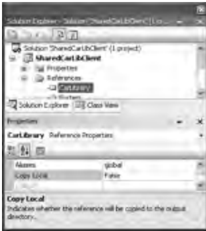
Figure 11-23. The Copy Local property can force a copy of a strongly named code library.
