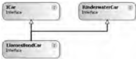
Figure 7-6. Multiple inheritance of interface types is allowed by the CTS.
