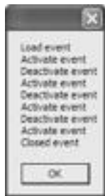
Figure 19-5. The life and times of a Form-derived type
