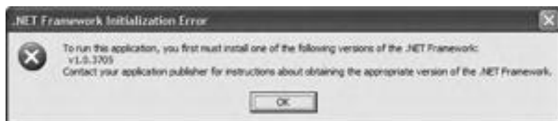
Figure 13-14. <requiredRuntime> results in a runtime error if the specified version of the CLR is not
