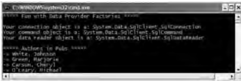
Figure 22-2. Obtaining the SQL Server data provider via the .NET 2.0 data provider factory
