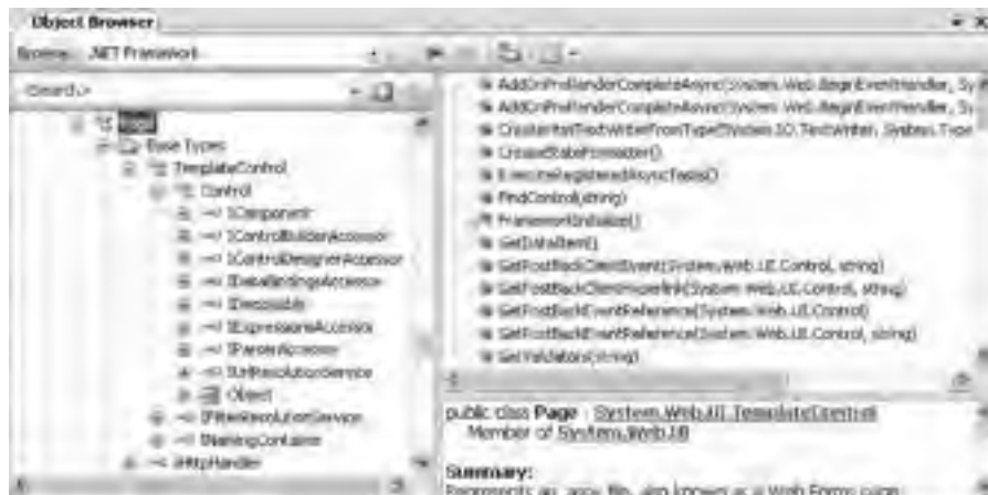
Figure 23-18. The derivation of an ASP.NET page
