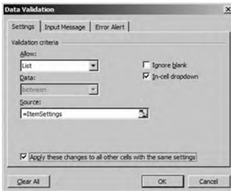
**Figure 20-6. Values from the validation list appear in a dropdown**
