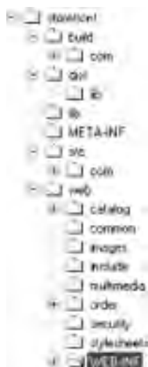
Figure 16-3. The build structure for the Storefront application
