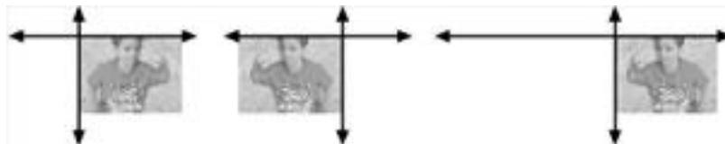
Figure 8-2. Matrix-based mirror image transformation steps: original, scaled by x-factor of -1, translated by adding width
