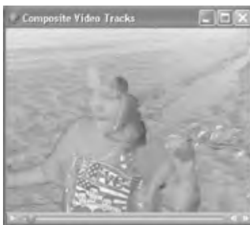
Figure 8-4. Composited video tracks with addMax graphics mode
