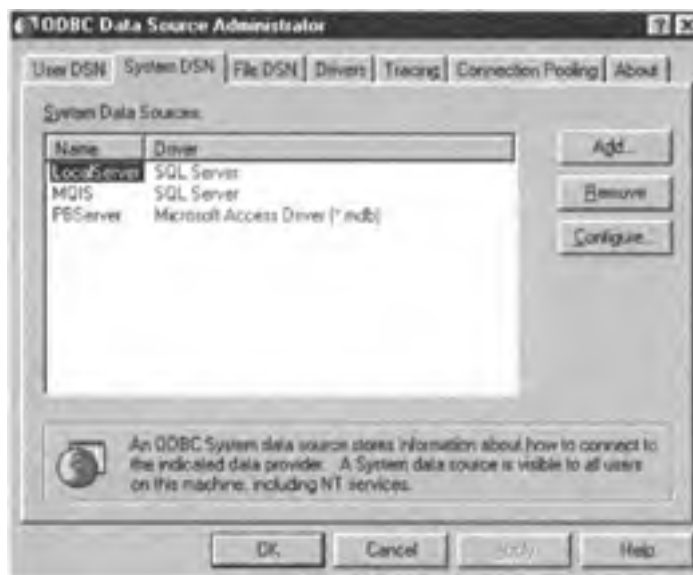
Figure 585.1: The System DSN tab within the ODBC Data Source Administrator Dialog box
