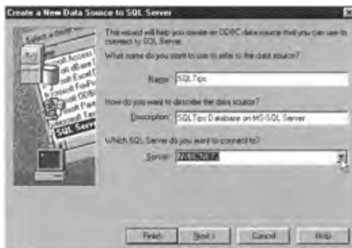
Figure 585.3: Screen 1 of the ODBC Data Source Administrator Create a New Data Source to SQL Server dialog box
