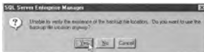
Figure 518.2: The MS-SQL Server Enterprise Manager message warning that folders in the backup device pathname do not exist or are not currently accessible
