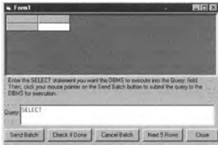
Figure 425.1: Visual Basic form with a text field to accept a user's dynamic SQL statement during runtime
