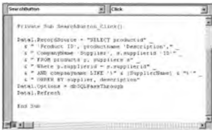
Figure 371.2: The code pane of the VB application window with the code for the CommandButton Control named SearchButton
