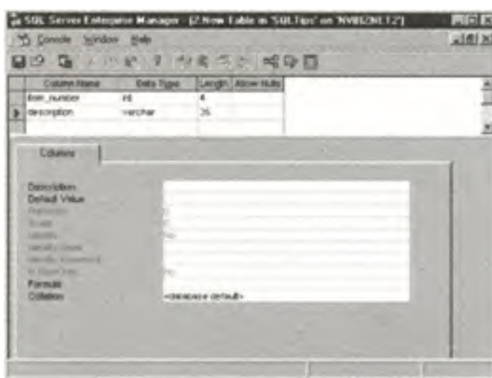
Figure 47.2: The MS-SQL Server Enterprise Manager New Table window after defining two columns for the ITEM_MASTER table
