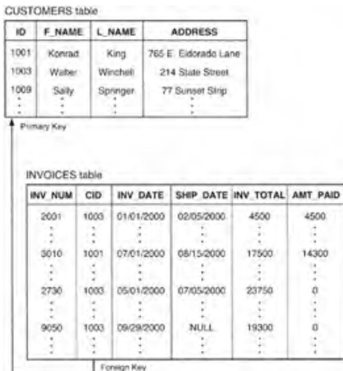
Figure 284.1: CUSTOMERS (parent) table and INVOICES (child) table related by common columns-ID in CUSTOMERS and INV_NUM in INVOICES
