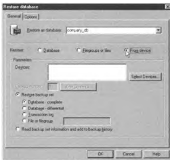
Figure 521.2: The MS-SQL Server Enterprise Manager Restore Database dialog box's General tab, with Restore from Device options displayed
