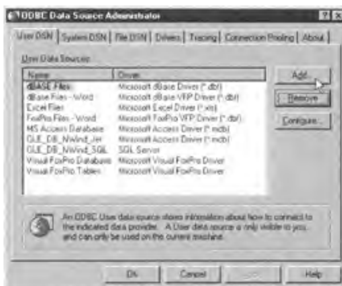
Figure 368.1: The User DSN tab of the ODBC Data Source Administrator dialog box
