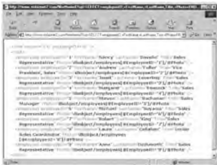
Figure 600.1: XML document displayed without an XSL style sheet as displayed by IE
