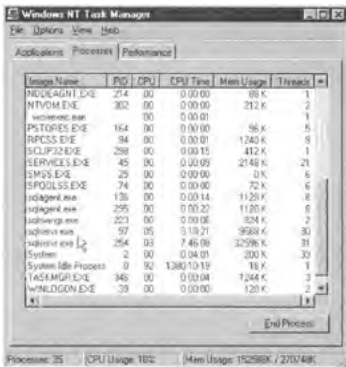
Figure 501.1: The Windows NT Task Manager showing statistics on processes running on an NT Server
