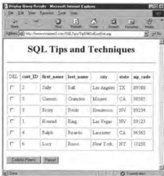
Figure 594.1: An HTML form that has a check box which displays the CUSTOMERS query results set and has a check box the user can use to mark customers for deletion
