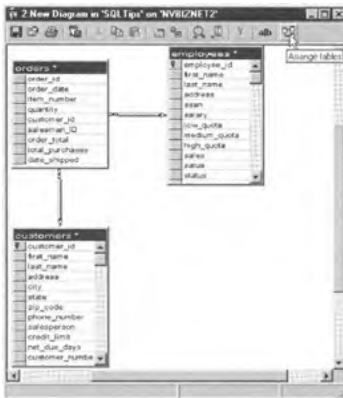
Figure 187.4: The Create Database Diagram Wizard New Diagram window, graphically depicting the FOREIGN KEY links between tables
