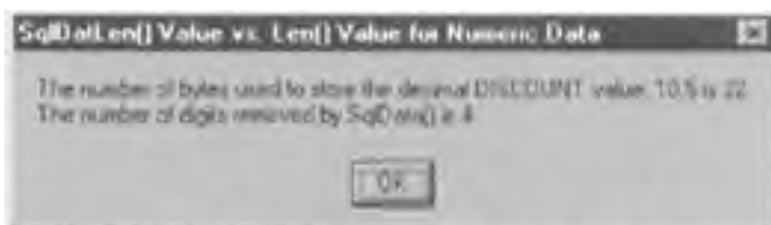
Figure 412.1: A Windows message box displaying the results of the SqlDatLen() and Len() function calls for numeric (decimal) data retrieved by an SqlData() function call
