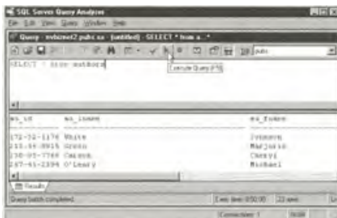
Figure 38.3: The Query Analyzer, with a query in the Query pane and query results in a Results pane
