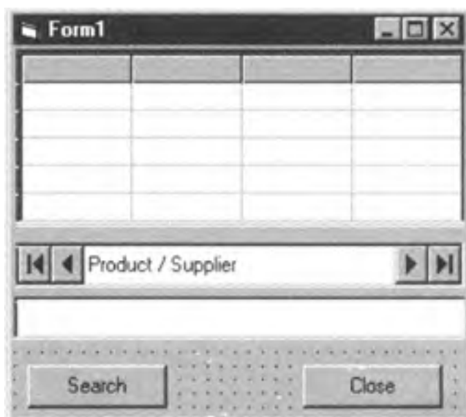
Figure 371.1: A VB SQL query form with a Data Control, an MSFlexGrid Control, a TextBox Control, and two CommandButton Controls
