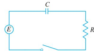
30. In the circuit of Exercise 29,  $R = 2 \Omega$ ,  $C = 0.01$  F,  $Q(0) = 0$ , and  $E(t) = 10 \sin 60t$ . Find the charge and the current at time  $t$ .
